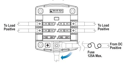
Application Note: This device is intended for branch circuit protection. Suitable main circuit protection of not more than 125A rating should be provided ahead of this device with an interrupt current rating consistent with the battery capacity. Consult ABYC E-11 Table V See "Circuit Protection" at www.bluesea.com.
