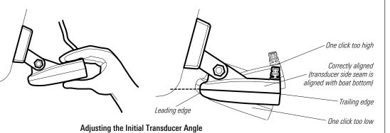
7. Adjust the transducer assembly vertically, until the seam on the leading edge of the transducer (the edge closest to the transom of the boat) is level and just slightly below the hull.
