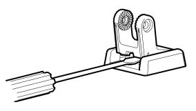
4. Align the mounting bracket transducer assembly with the drilled holes in the transom. With a 5/16" socket driver, mount the assembly to the transom using the two #10 - 1" long screws (provided). Hand tighten only!
