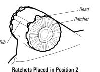
Fitting the Mounting Bracket Over the Ratchet
