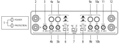
1. Status LEDs (on top of amplifier): Power and Protection—Power will illuminate to indicate the amplifier is on and operating normally; protection will illuminate if the amplifier shuts down due to short circuit, DC offset, or overheating detected by onboard protection circuitry.
