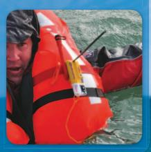
Easy activation – just slide off the orange arming tab, then pull off the red activation cap
