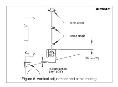
such as trim tabs, pumps or wiring inside the hull. Mark the location with a pencil. Drill a hole using the appropriate size bit to accommodate the connector.
