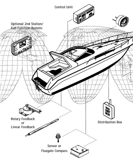
A basic ComNav 1001 electronics package includes: Control Unit, Distribution Box, Fluxgate Compass or Standard Sensor for a Magnetic Compass, output for Solenoid Valves, Rotary or Linear Feedback and Interconnecting Cables.
