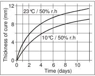
Diagram 1: Curing speed Sikaflex®-295 UV
