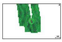
A green circle indicates good depth and GPS position, and a speed under 16 km/h (10 mph). A yellow circle indicates good depth and GPS position, and a speed between 16 and 32 km/h (10 and 20 mph). A red circle indicates poor depth or GPS position, and a speed above 32 km/h (20 mph).
