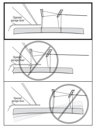
**DIAGRAM 1.** Plan to position object above car with clearance to open garage door. If Hoister is mounted too close to garage door, there may not be clearance to open door. Mounted too far forward, object may not balance or lower onto car.
