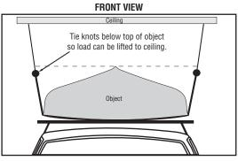
**DIAGRAM 26.** Tie knots below top of object so object can be lifted to ceiling. Adjust strap length in buckle as needed.
