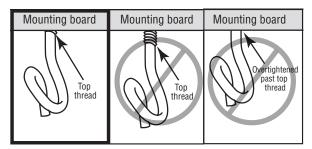
**DIAGRAM 7.** Install a pigtail lag screw (B) in each hole. Threads should disappear into mounting board.
