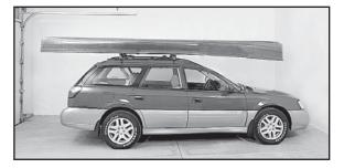
Measure length of object. Plan to position Hoister so garage door can open with object lowered.
