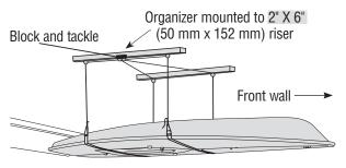
Use 2" X 6" (50 mm x 152 mm) mounting boards. Mount the organizer on a 2" X 6" X 7" (50 mm x 152 mm x 180 mm) riser board.
