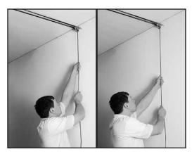
With rope pointed down, the cleat will lock the rope. Angle to release. Repeat until object is at desired height.
