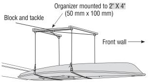
Mount pigtail lag screws to 2" X 6" (50 mm x 152 mm) mounting boards similar to Diagram 16 (page 13), except block and tackle goes to side wall of garage. Use a 2" X 4" (50 mm x 100 mm) as shown to mount the organizer.
