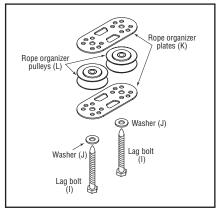
**DIAGRAM 19.** Assemble rope organizer as shown in Diagram 17 using plate (K) and pulleys (L). Fasten to  $2" \times 4"$  (50 mm x 100 mm) with lag bolts (I) and washers (J).
