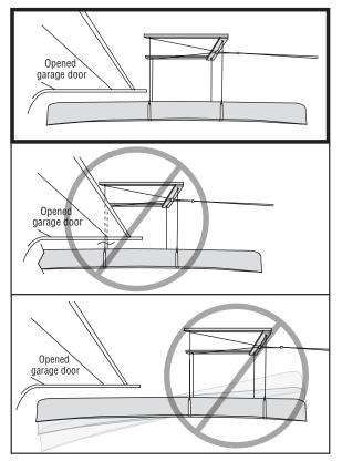
**DIAGRAM 13.** Plan to position object above car with clearance to open garage door. If Hoister is mounted too close to garage door, there may not be clearance to open door. Mounted too far forward, object may not balance or lower onto car.
