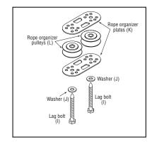
**DIAGRAM 10.** Assemble rope organizer using plate (K) and pulleys (L). Fasten to mounting board with lag bolts (I) and washers (J).
