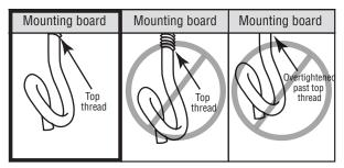
**DIAGRAM 18.** Install a pigtail lag screw (B) in each hole. Threads should disappear into mounting board.
