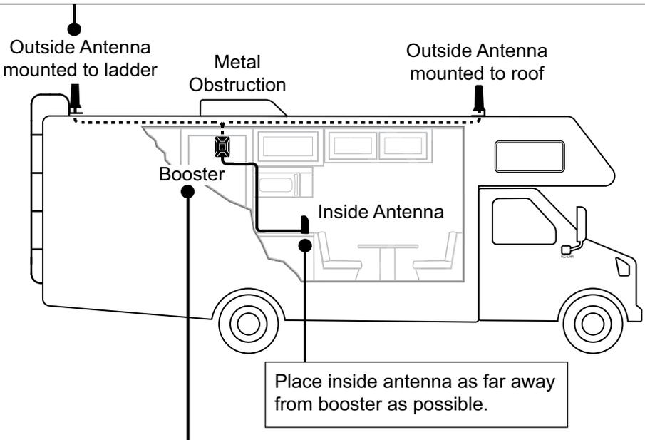
Mount booster as far away from outside antenna as possible, but make sure 20 foot cable will still reach between the two.
