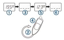
**6** Within three minutes, complete two full, slow, tight circles ②, taking care to keep the boat as steady and level as possible. Heading data disappears to indicate that the antenna has detected the start of the procedure ③.
