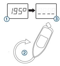
**6** Within three minutes, complete two full, slow, tight circles ②, taking care to keep the boat as steady and level as possible. The boat should not list during calibration.
