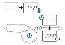
When the heading data appears, the compass has been calibrated successfully, and you can align the heading (optional).
