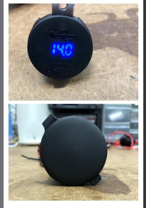
USB PM2 has translucent cover to allow battery voltage to be monitored even when not in use. As compared to the USB PM
