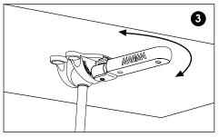
IMPORTANT: Make sure that the handle is tightened fully.
